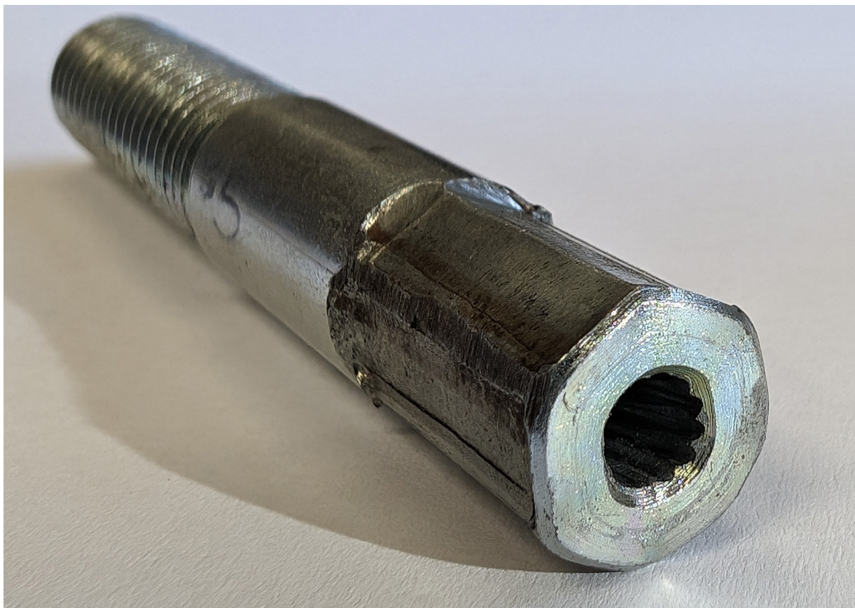
Figure 11: Termination piece which was crimped onto the handbrake cable to allow it to connect to the pivots.
