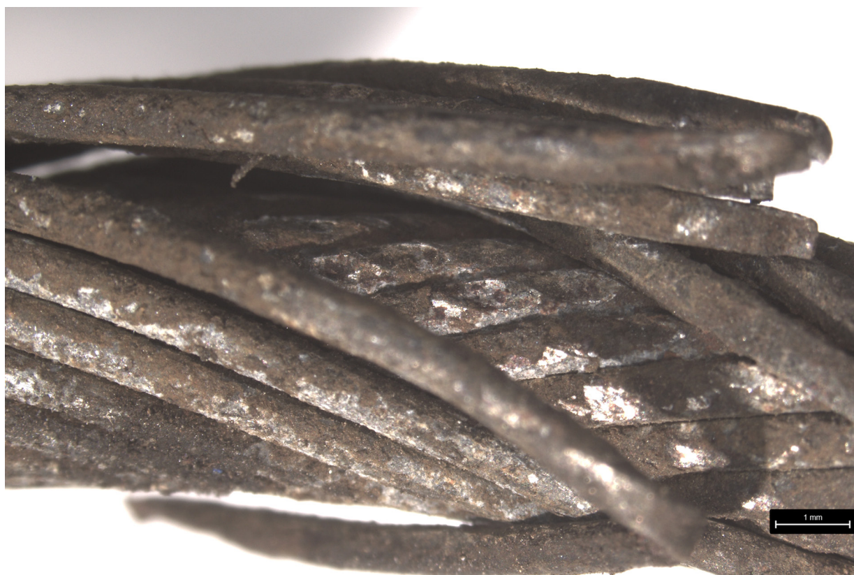
Figure 12: Deformation of the individual cable strands caused by the cable crushing itself due to high tensile loads.
