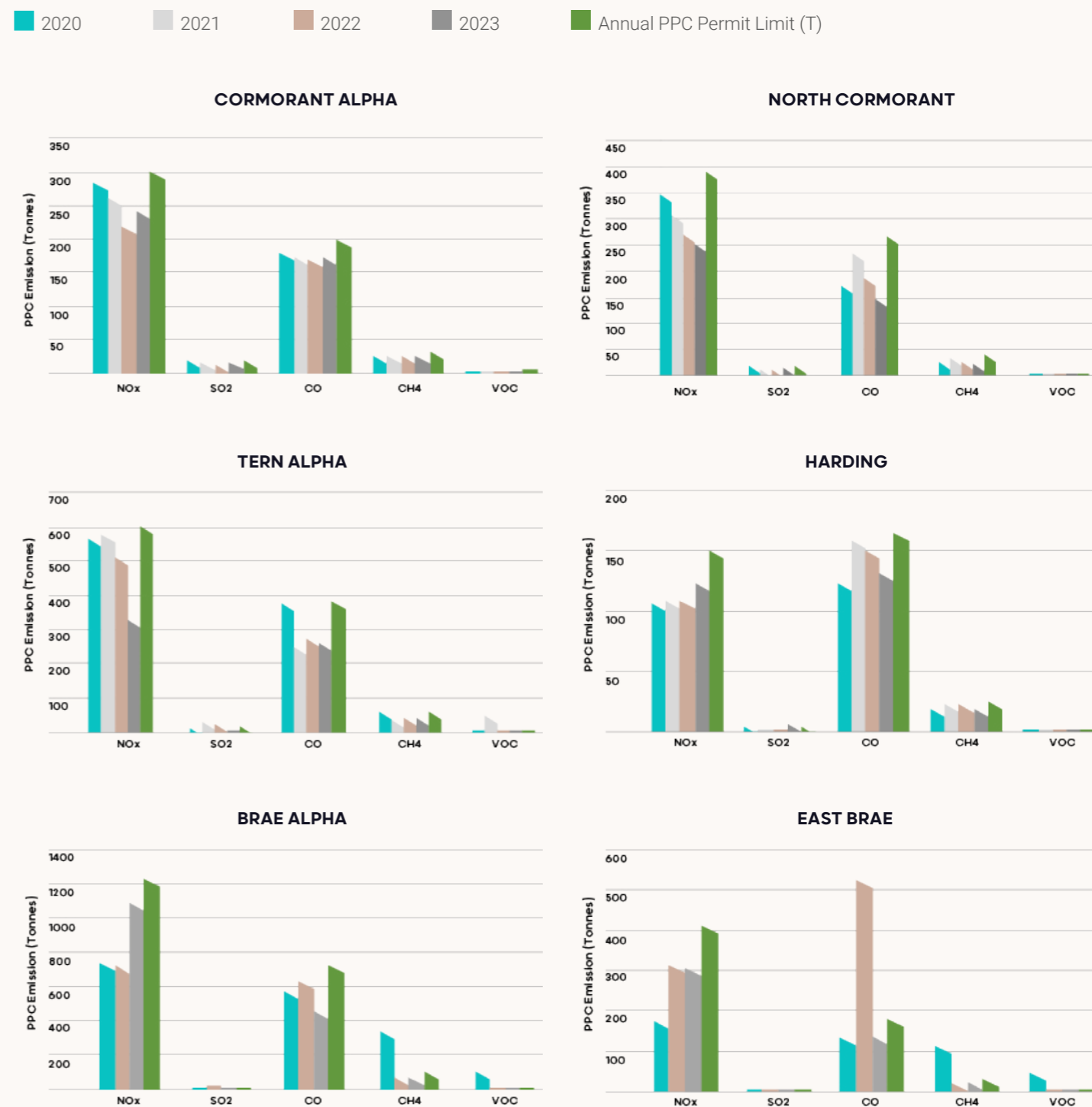
FIGURE 2 TAQA UK’S ACTUAL NON- CO 2 ATMOSPHERIC EMISSIONS VERSUS PERMIT ALLOWANCE
