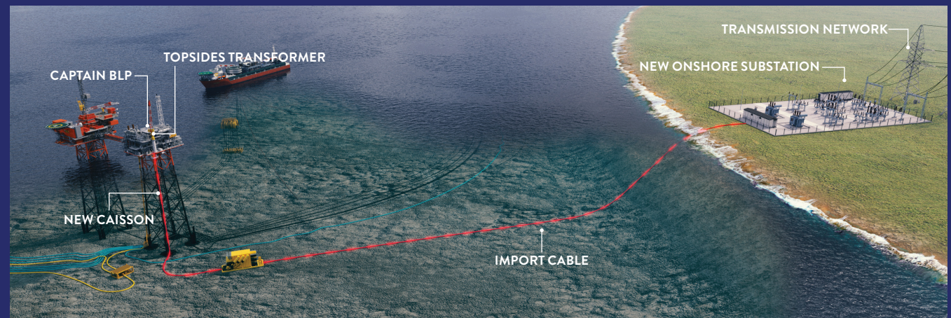
Fig – FEED graphic of potential Captain electrification option showing shore tie-in and new subsea cable, caisson and topsides equipment.
