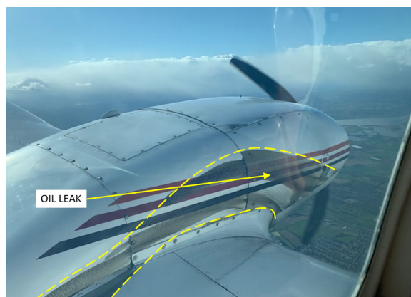
Photograph taken in-flight of the oil leak from the left engine
