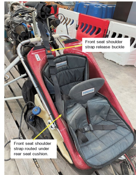
Front seat diagonal shoulder strap positioned as found at the accident site
