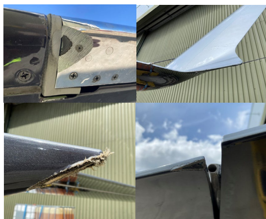
Damage to LX-NST. Clockwise from top left – slat, winglet, aileron, flap fairing
