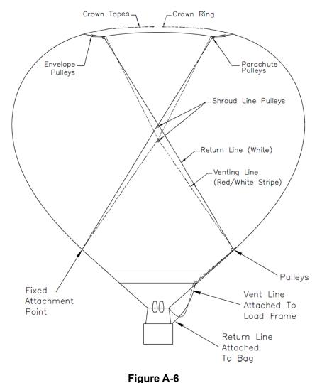
Schematic of the Para Plus venting and deflation system
