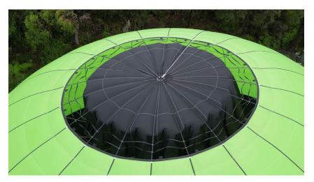
**Figure A-4** Picture of Lite Vent showing vent edges rolled inwards.
