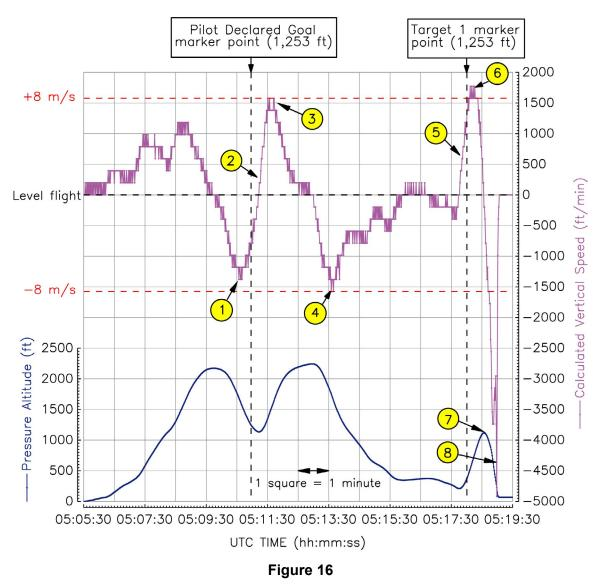
Altitude (blue) and vertical speed (purple) profile of the accident flight
