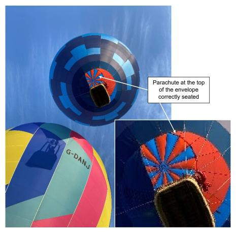
Figure 4 G-CMFS just after launch showing the parachute correctly seated
