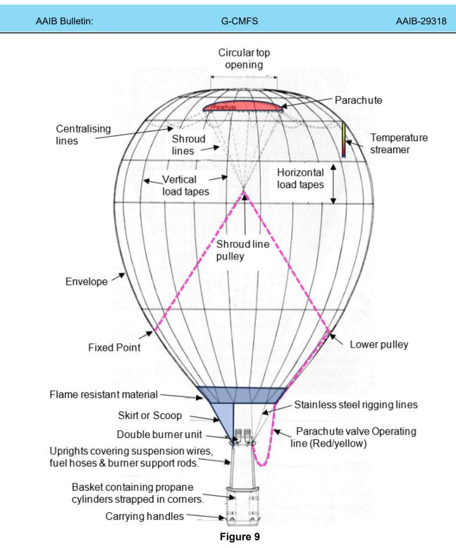
Basic features of a generic racing balloon showing internal rigging arrangements
