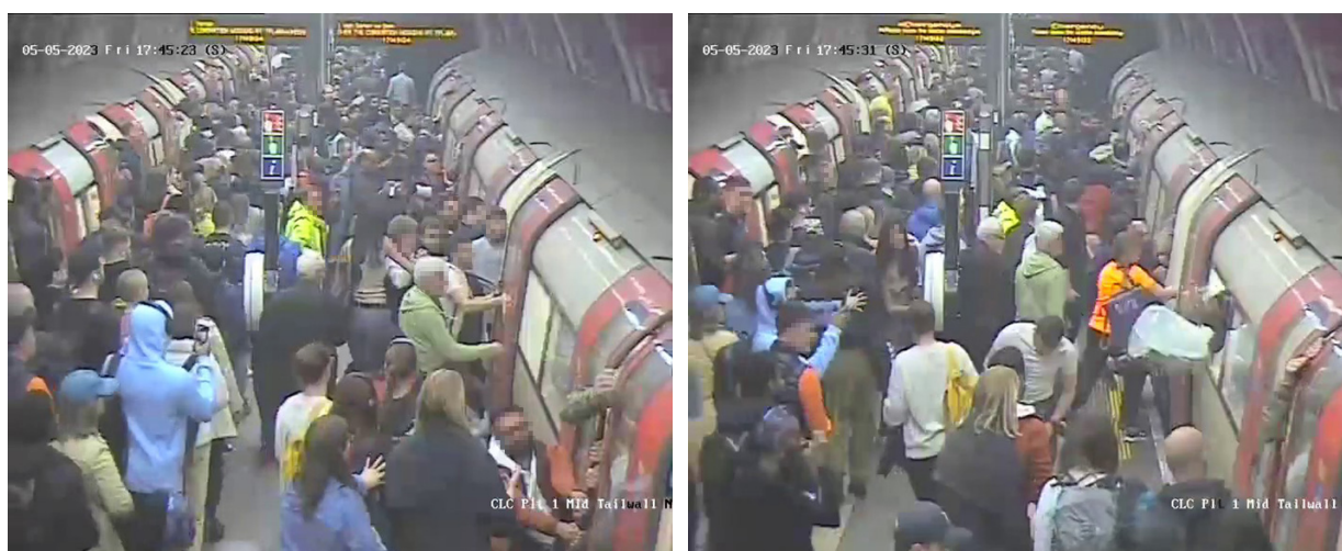
Figure 1: Closed-circuit television (CCTV) footage from Clapham Common station platform at 17:45 hrs; the camera is facing towards the steps leading to the platform. Left-hand image shows a passenger breaking a bodyside window on car 5 of train 065 and right-hand image shows passengers beginning to evacuate from the train via the broken window (courtesy of LUL).
