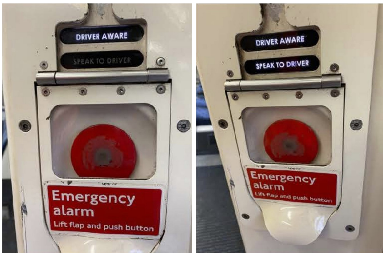
Figure 8: PEA system alarm on 1995 stock. Once activated the 'Driver Aware' sign will light up (left-hand side image). When the train operator answers the PEA the 'Speak to Driver' sign illuminates (right-hand side image) allowing the passenger to communicate with the train operator. Courtesy of LUL.
