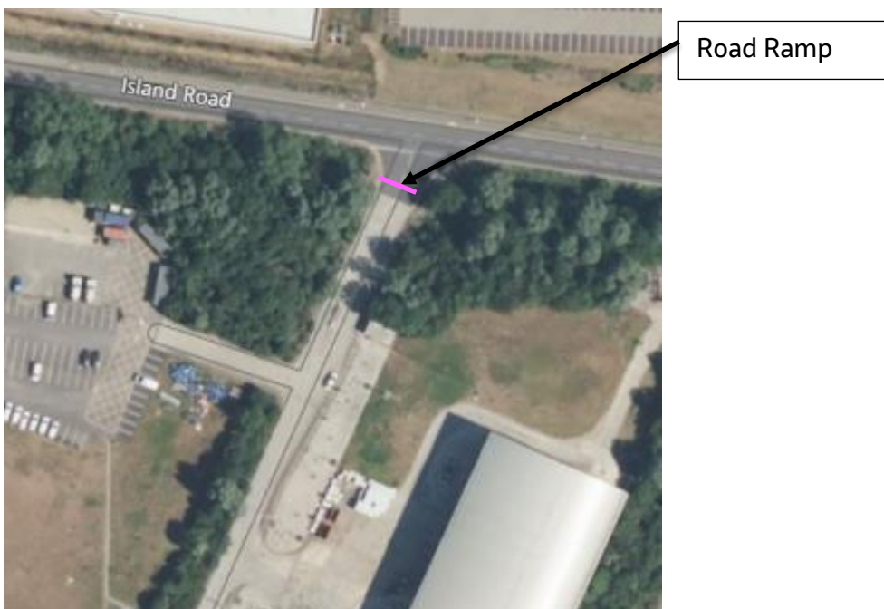
Figure 4.4 – Road Ramp for tertiary containment
