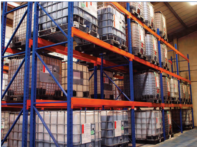
Figure 3.1 Typical storage of IBCs in a warehouse (courtesy Feedwater Ltd)
