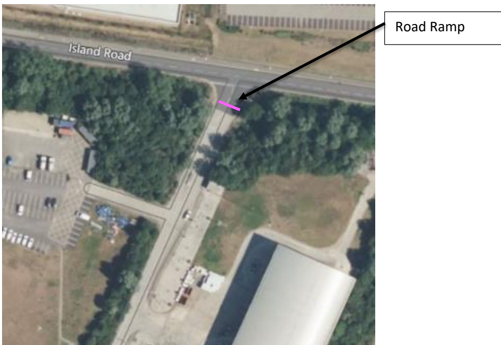
Figure 4.4 – Road Ramp for tertiary containment
