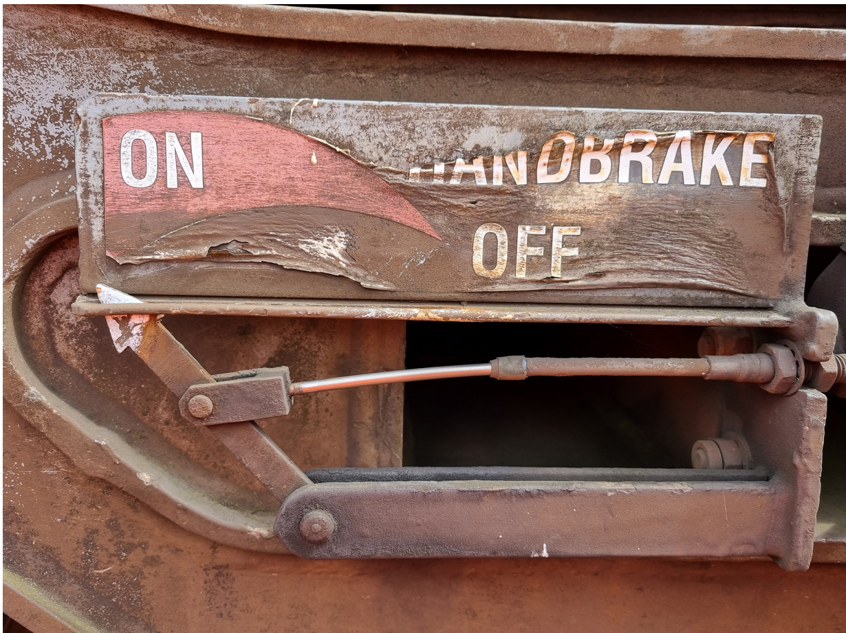
Figure 15: Handbrake indicator from an FAA wagon.
