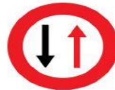
Priority to oncoming vehicles (Red arrow indicated need to yield to oncoming vehicles)
