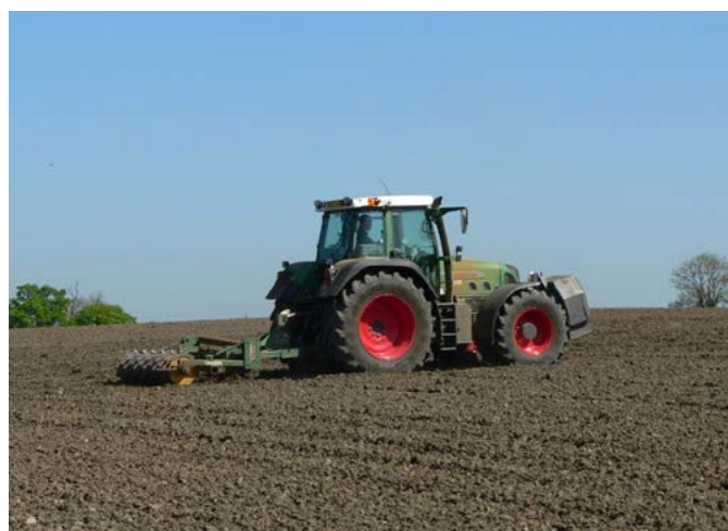
A tractor in a bare field towing a machine that is performing sub-soiling.
