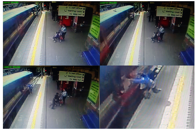
Passenger trapped in closing doors and dragged along the platform at Hayes & Harlington.
