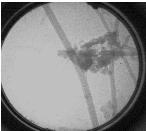
Fig 2e: Example of particle attached to chrysotile fibres. An example of the characteristic tubular structure of chrysotile can be seen. Any significant change to the chemistry is likely to be reflected by the tubular structure being broken down.
