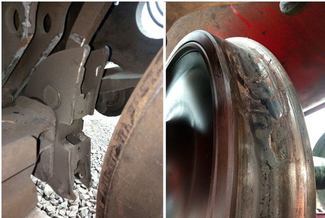
Missing components and damaged wheel treads following locking of a wagon brake mechanism.
