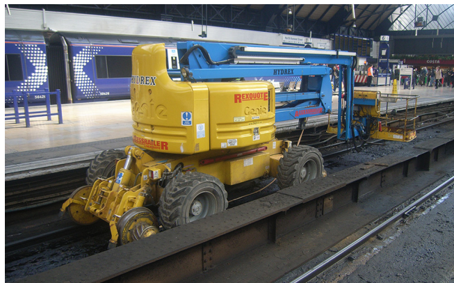
RRV after running away into Glasgow Queen Street station.
