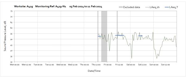
Note: Missing data from the start of the month until 14:00 on Thursday 8<sup>th</sup> February was due to loss of power to the monitoring station. The monitoring station battery and battery connectors were replaced with view of minimising loss of data in the future.
