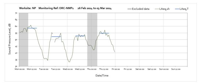
Note: Missing data between 10:00 and 11:00 on Tuesday 27<sup>th</sup> February was due to a communication error between the monitoring station and server.
