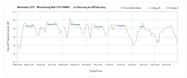
Note: Missing data between 23:00 and 00:00 on Tuesday 13<sup>th</sup> February was due to a communication error between the monitoring station and server.
