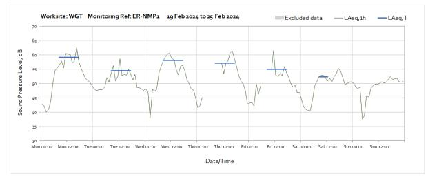
Note: Missing data throughout the week was due to a loss of power to the monitoring station caused by poor weather conditions preventing sufficient light to reach the solar panel.
