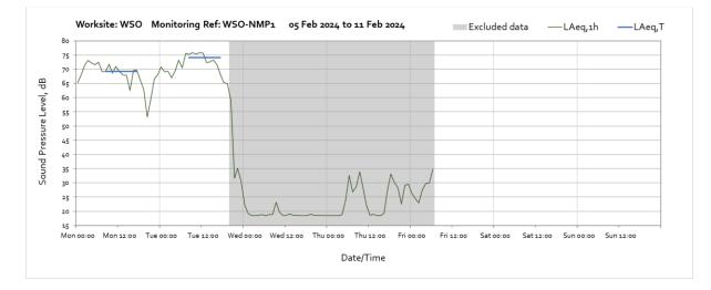
Note: Missing data from 07:00 on Friday 9th February until month end was due to water ingress to monitor from flooding, area is currently inaccessible to allow installation of dewatering pump.
