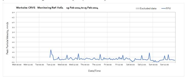
Note: Missing data from 16:00 on Thursday 15<sup>th</sup> until 11:00 on Tuesday 20<sup>th</sup> February was due to loss of power to the monitoring station caused by a depleted battery.
