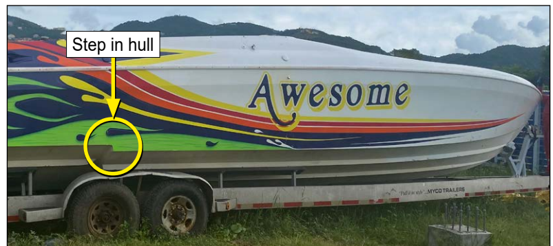
Figure 9: Pressure zone on a stepped planing hull and step in Awesome's hull
