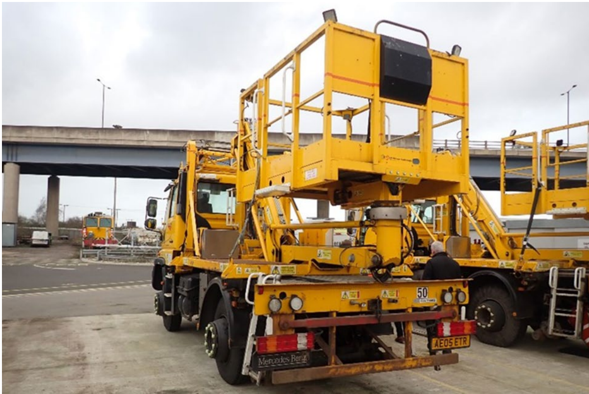
A Network Rail road-rail vehicle with a mobile elevated work platform and basket as used on the East Coast Main Line for overhead line equipment inspections.
