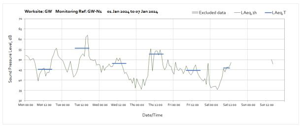
Note: Missing data throughout the week was due to loss of power at monitoring station caused by poor weather conditions preventing sufficient light to reach the solar panel.
