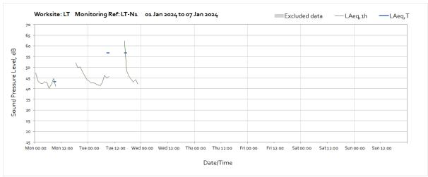
Note: Missing data throughout the week was due to loss of power at monitoring station caused by poor weather conditions preventing sufficient light to reach the solar panel.
