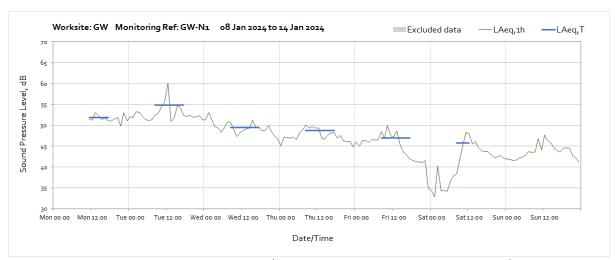
Note: Missing data between 17:00 on Sunday 7<sup>th</sup> of January 2024 until 10:00 on Monday 8<sup>th</sup> of January 2024 was due to loss of power at monitoring station caused by poor weather conditions preventing sufficient light to reach the solar panel.
