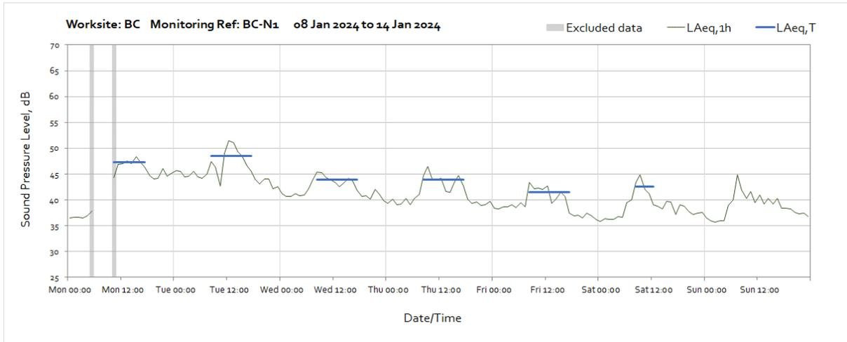
Note: Missing data from 08<sup>th</sup> of January at 06:00 until 09:00 was due to a loss of power at the monitoring station caused by insufficient sunlight for the solar panels.
