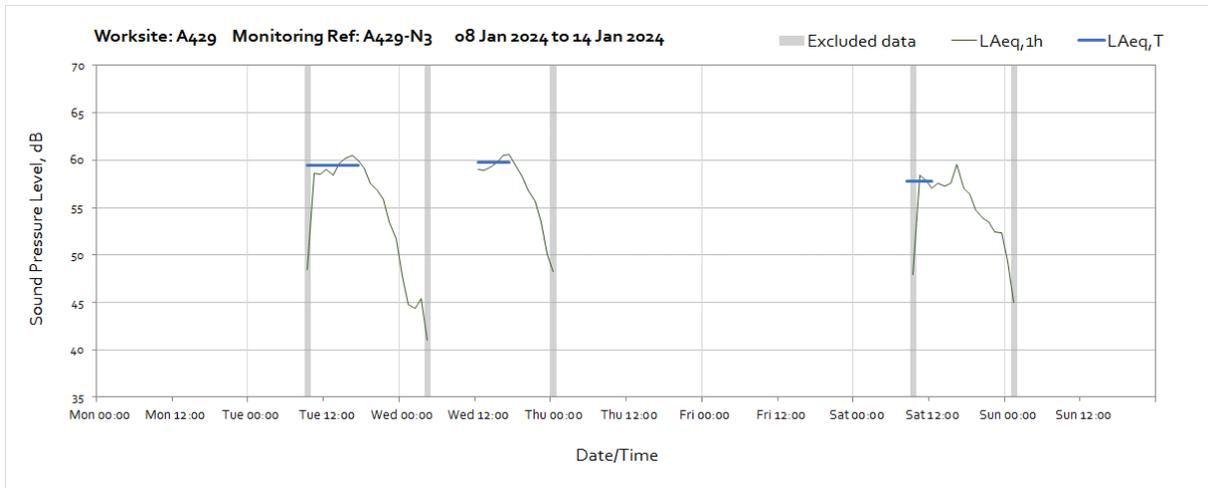
Note: Missing data throughout the week was due to a loss of power at the monitoring station caused by insufficient sunlight for the solar panels.
