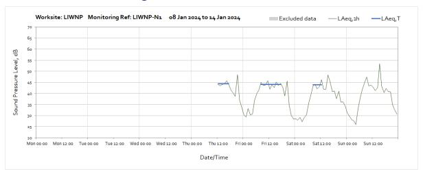
Note: Missing data from the beginning of the month until 12:00 on Thursday 11<sup>th</sup> January was due to a loss of power to the monitoring station caused by depletion of battery power, which has since been replaced.
