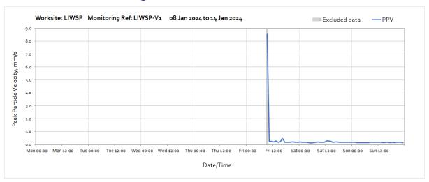
Note: Missing data from the beginning of the month until 09:00 on Friday 12<sup>th</sup> January was due to a loss of power to the monitoring station caused by poor weather conditions preventing sufficient light from reaching the solar panel.
