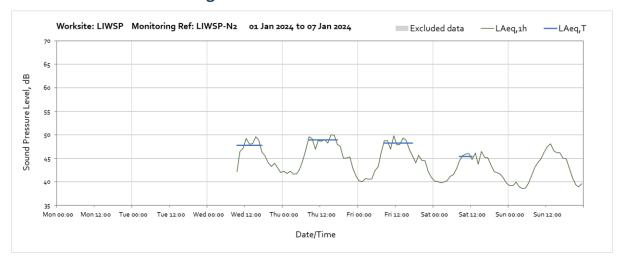
Note: Missing data from the beginning of the month until 09:00 on Wednesday 3<sup>rd</sup> January was due to a loss of power to the monitoring station caused by poor weather conditions preventing sufficient light from reaching the solar panel.
