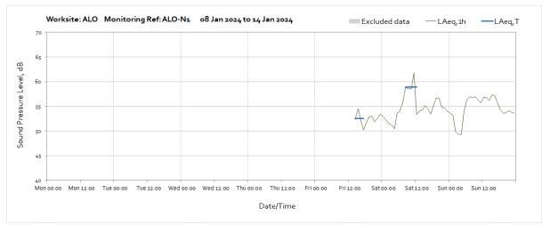
Note: Missing data from the beginning of the month until 14:00 on Friday 12<sup>th</sup> of January was due to the loss of power at the monitoring station caused by poor weather conditions preventing sufficient light to reach the solar panel.
