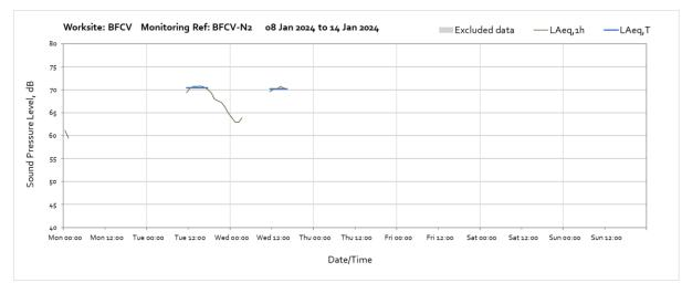
Note: Missing data throughout the week was due to the loss of power at the monitoring station caused by poor weather conditions preventing sufficient light to reach the solar panel.
