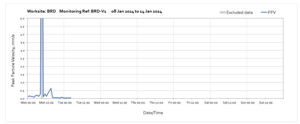
Note: Missing data between 04:00 on Tuesday 9<sup>th</sup> and 14:00 on Thursday 25<sup>th</sup> January was due to the loss of power at the monitoring station caused by connection issues between the power source and the monitoring station.
