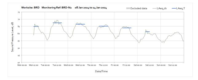
Note: Missing data throughout the first week of the month until 12:00 on Monday 8<sup>th</sup> of January was due to the loss of power at the monitoring station caused by poor weather conditions preventing sufficient light to reach the solar panel.
