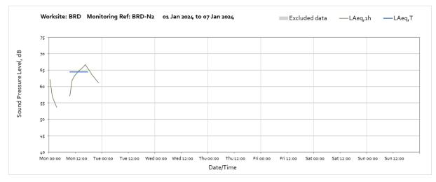
Note: Missing data throughout the first week of January was due to the loss of power at the monitoring station caused by poor weather conditions preventing sufficient light to reach the solar panel.
