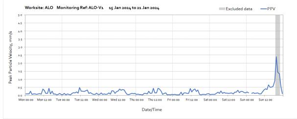
Note: Missing data between 02:00 and 03:00 on Sunday 21<sup>st</sup> January was due to the loss of power at the monitoring station caused by poor weather conditions preventing sufficient light to reach the solar panel.
