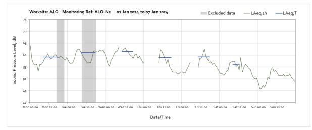
Note: Missing data throughout the week was due to the loss of power at the monitoring station caused by poor weather conditions preventing sufficient light to reach the solar panel.
