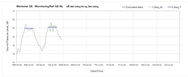
Note: Missing data from 22:00 on Tuesday 9<sup>th</sup> January until the end of the month was due to the loss of power at the monitoring station caused by the disconnection of mains power.
