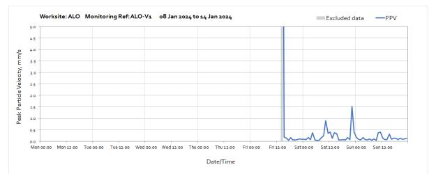
Note: Missing data from the beginning of the month until 14:00 on Friday 12<sup>th</sup> January was due to the loss of power at the monitoring station caused by poor weather conditions preventing sufficient light to reach the solar panel.
