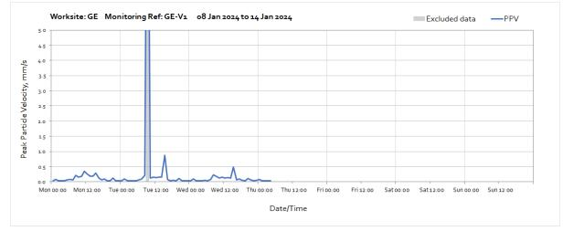
Missing data from 04:00 on Thursday 11<sup>th</sup> January until the end of the month was due to the loss of power at the monitoring station caused by the disconnection of mains power.
