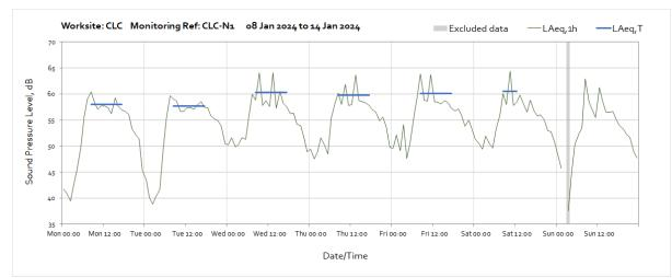
Note: Missing data between 01:00 and 03:00 on Sunday 14<sup>th</sup> of January was due to a clock synchronization error at monitoring station.
