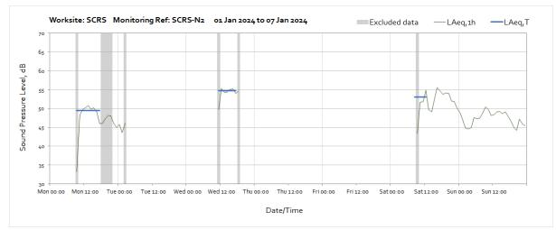
Note: Missing data throughout the week was due to poor weather conditions preventing sufficient light from reaching the solar panel.
