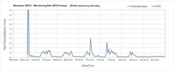
Note: Missing data between 17:00 on Saturday 6<sup>th</sup> January and 15:00 on Monday 8<sup>th</sup> January was due to a loss of power to the monitoring station caused by poor weather conditions preventing sufficient light reach the solar panel.
