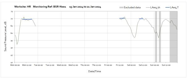
Note: Missing data between 22:00 on Monday 15<sup>th</sup> January and 12:00 on Friday 19<sup>th</sup> January was due to a loss of power to the monitoring station caused by poor weather conditions preventing sufficient light to reach the solar panel.
