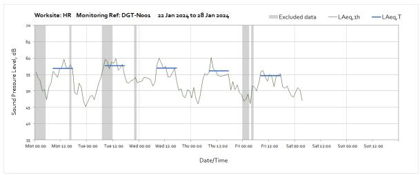
Note: Missing data from 04:00 on Saturday 27<sup>th</sup> January until the end on the month was due to a loss of power to the monitoring station caused by poor weather conditions preventing sufficient light to reach the solar panel.
