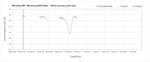
Note: Missing data throughout the week was due to a loss of power to the monitoring station caused by poor weather conditions preventing sufficient light to reach the solar panel.
