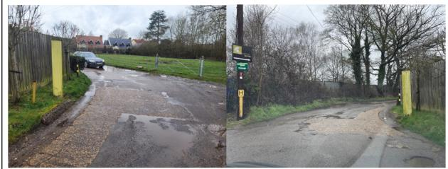
A give-way marking is proposed to delineate the extent of the site access, at a bend in Mill Lane. It appears that this give-way line is south of the existing carriageway edge and may reduce the width at the bend. Any large vehicle associated with the businesses to the north of the site may not be able to negotiate the new bend alignment and may overrun the give-way line, causing a collision with waiting vehicles.
