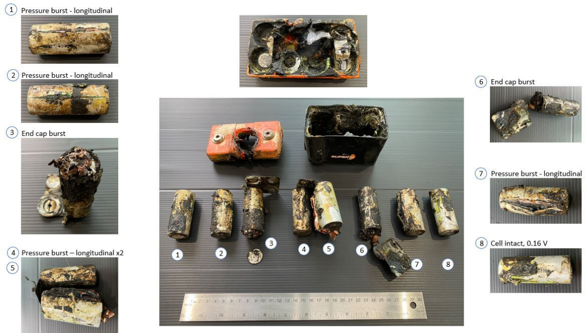
Figure 4 Damaged parts of the battery
