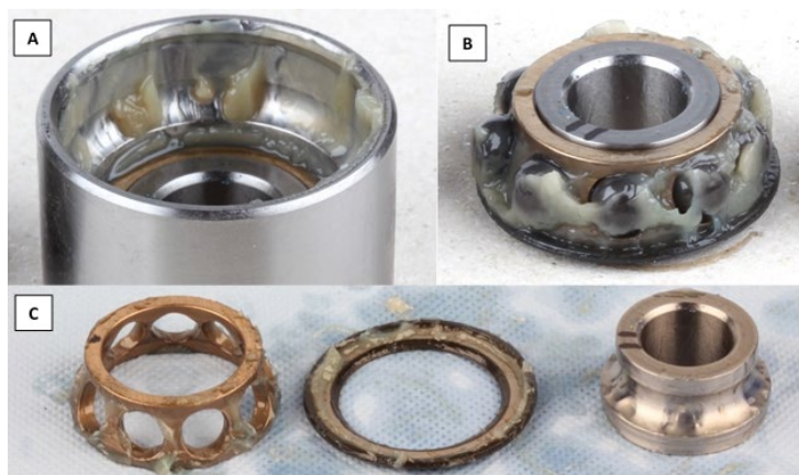
Bearing in new condition - (A) Housing and outer race, (B) inner race, cage and balls assembled, (C) cage, seal and inner race disassembled
