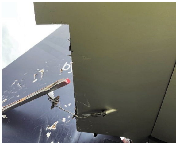
G-ZXEL lower side of right elevator showing trim tab detached at the hinge points but still connected via the control cables
