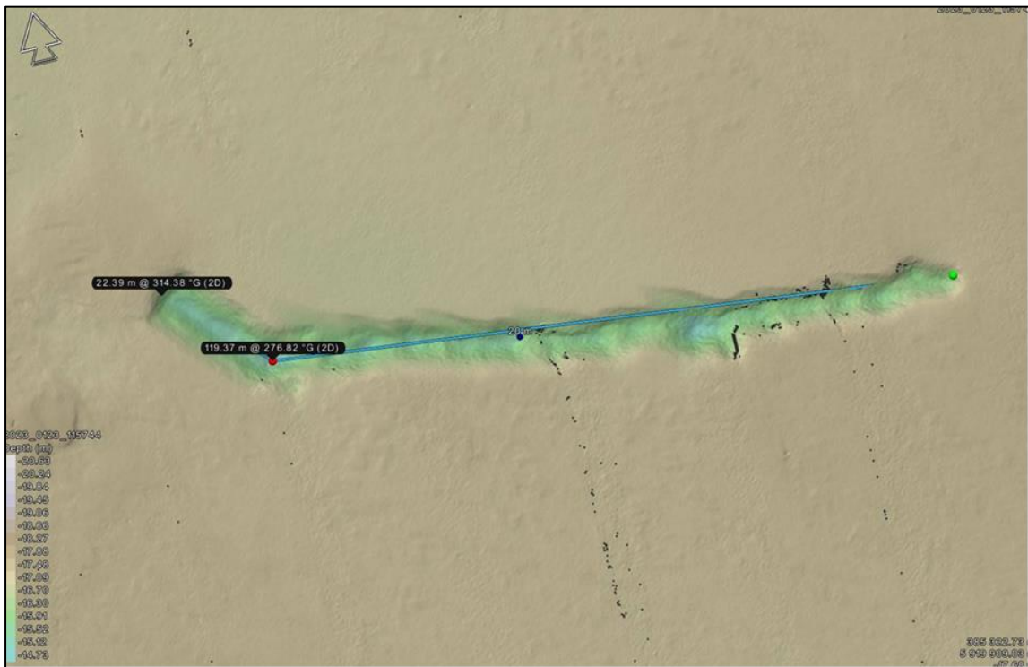
Figure 7-1: Historical rock placement on PL874/PL875 within the Guinevere 500m safety zone.
