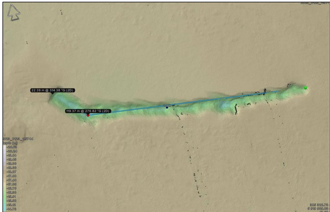
Figure 3-3: Historical rock placement on PL874/PL875 within the Guinevere 500m safety zone.
