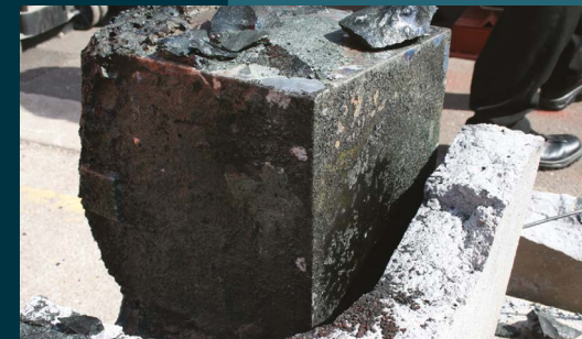
Product produced from Sellafield 2011 Geomelt Intermediate Level Waste Vitrification trials.
