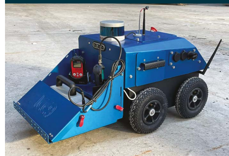
CARMA the autonomous radiation surveying robot with alpha, beta and gamma detectors attached. Credit to Manchester University
