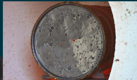
Close up showing drum structure failing during drum skid durability and structural integrity testing at high temperatures.
