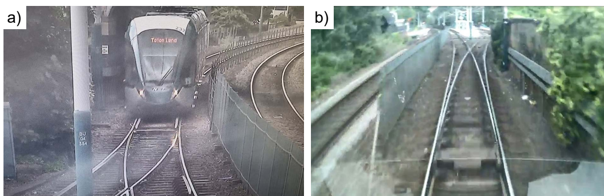
Figure 8: Still images from CCTV on a) Bulwell tram stop and b) tram 232 showing the state of BUP3 points immediately before tram 232 travelled over them. (Images courtesy of Nottingham Trams Ltd).
