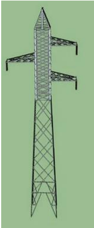
Figure 14 – Example of 110 kV transmission towers
