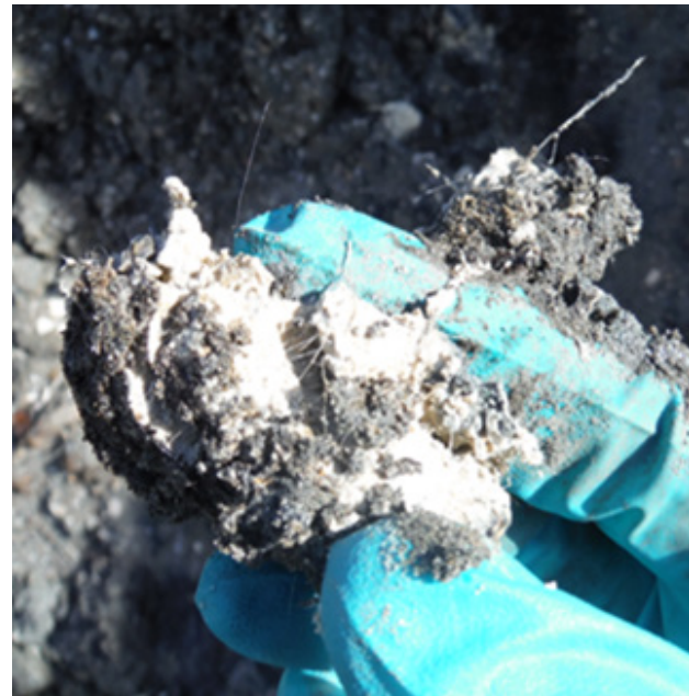
Degraded asbestos debris in soil | AECOM
