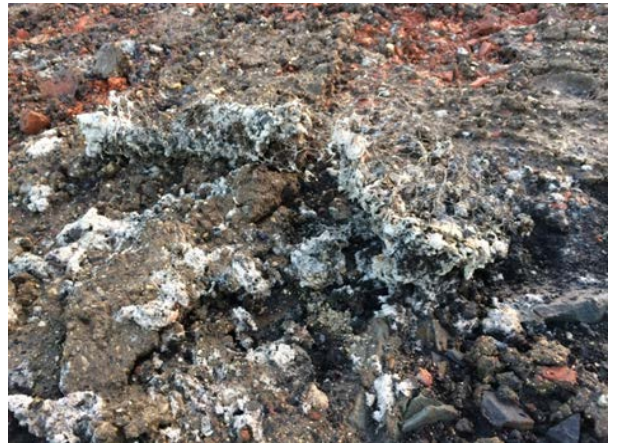
Photo courtesy of Soilfix Limited. Plate 28. Gross contamination of made ground by asbestos thermal insulation debris in 'chicken wire'.
