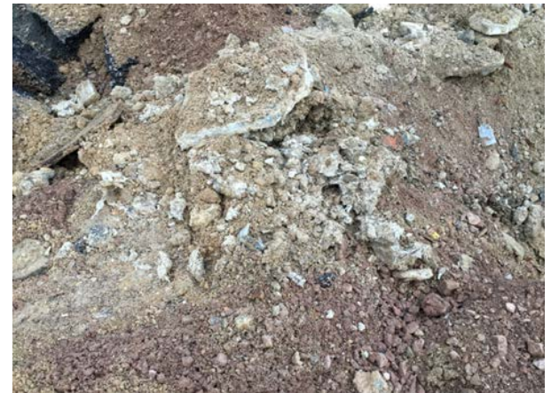
Photo courtesy of Hydrock. Plate 36. Highly degraded/disaggregated asbestos insulation/fibrous debris in excavated made ground.
