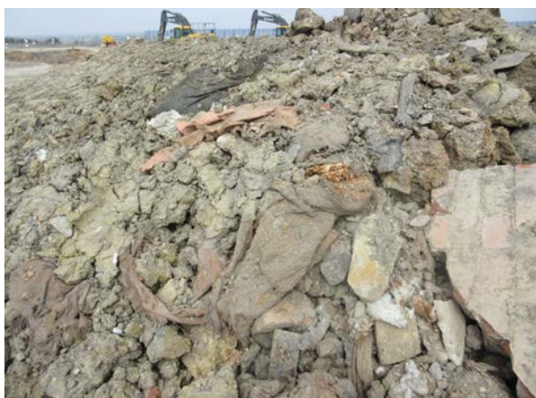
Photo courtesy of Hydrock. Plate 15. Weathered asbestos textile blankets in excavated made ground.
