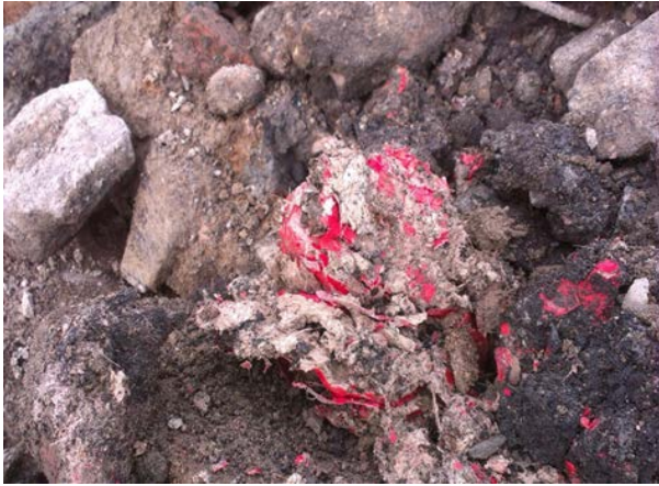
Photo courtesy of Soilfix Limited. Plate 25. Close-up of red-coated fibrous asbestos insulation debris.
