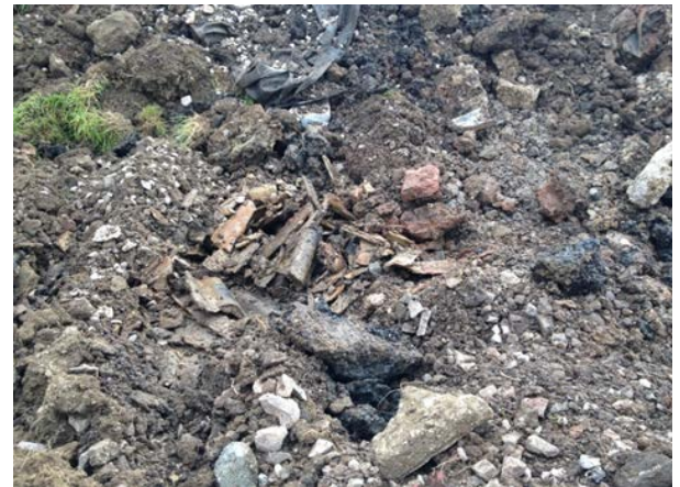
Photo courtesy of Soilfix Limited. Plate 10. Example of weathered asbestos cement debris in excavated made ground.
