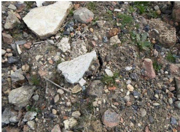
Photo courtesy of Hydrock. Plate 21. Degraded AIB/fibrous board on surface of made ground.
