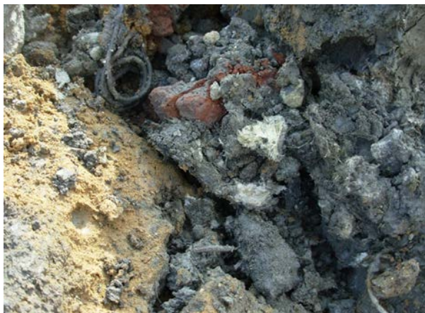
Photo courtesy of Soilfix Limited. Plate 29. Contamination of made ground by asbestos thermal insulation/fibrous debris.
