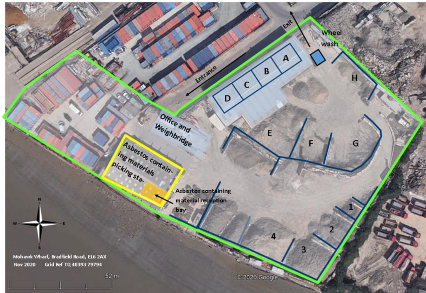
Figure 1. Plan of Mohawk to show Bay layout and location of Picking Station building
