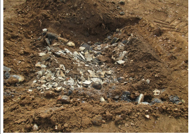
Photo courtesy of VertaseFLI. Plate 2. Pit containing degraded asbestos cement fragments and free fibres.
