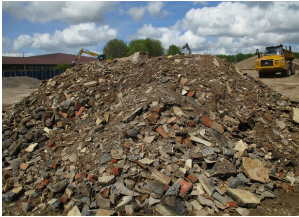
Photo courtesy of VertaseFLI. Plate 1. Extreme example of intact asbestos cement containing chrysotile in excavated made ground.
