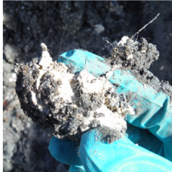
Degraded asbestos debris in soil | AECOM
