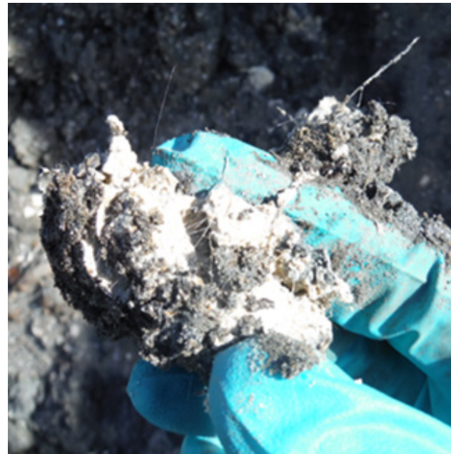
Degraded asbestos debris in soil | AECOM
