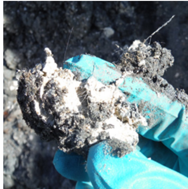
Degraded asbestos debris in soil | AECOM
