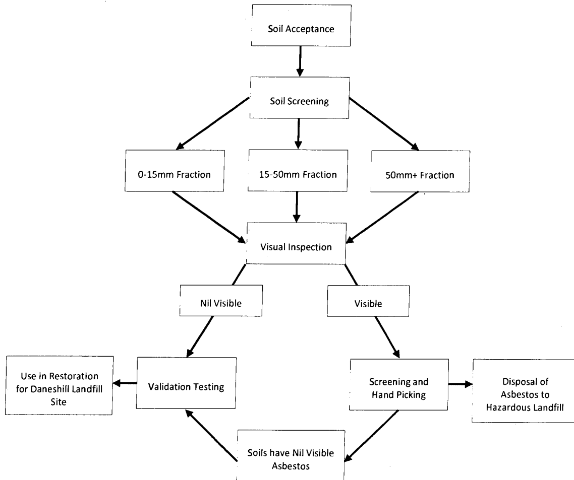
Figure 2: Overall Soil Treatment process at Daneshill Landfill Site
