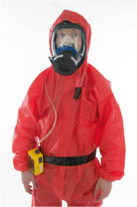
Figure 5.1 Removal worker wearing a personal pump
