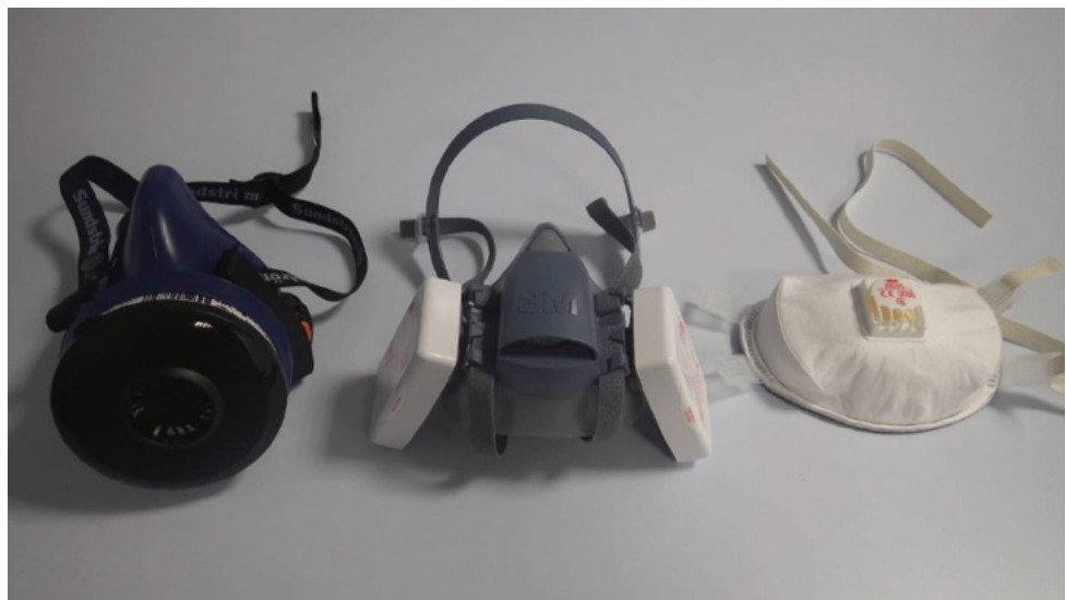
Figure 8.1 Types of filtering half-mask respirators
