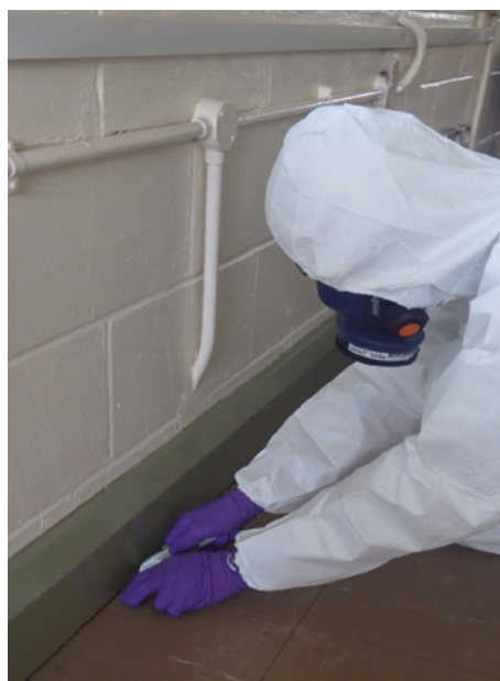
Figure 4.2 Sampling of a floor tile
