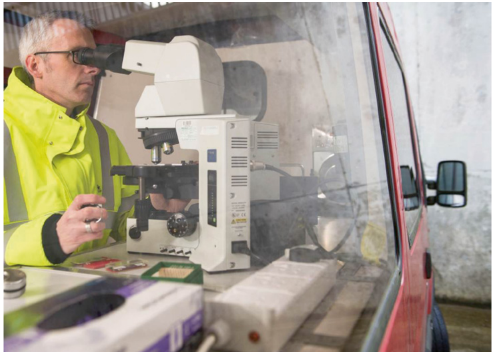
Figure 5.3 Analyst carrying out analysis by phase contrast microscopy in a mobile laboratory
