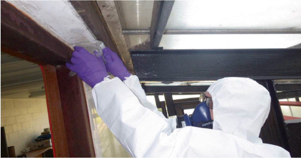
Figure 4.3 Sampling of AIB panels
