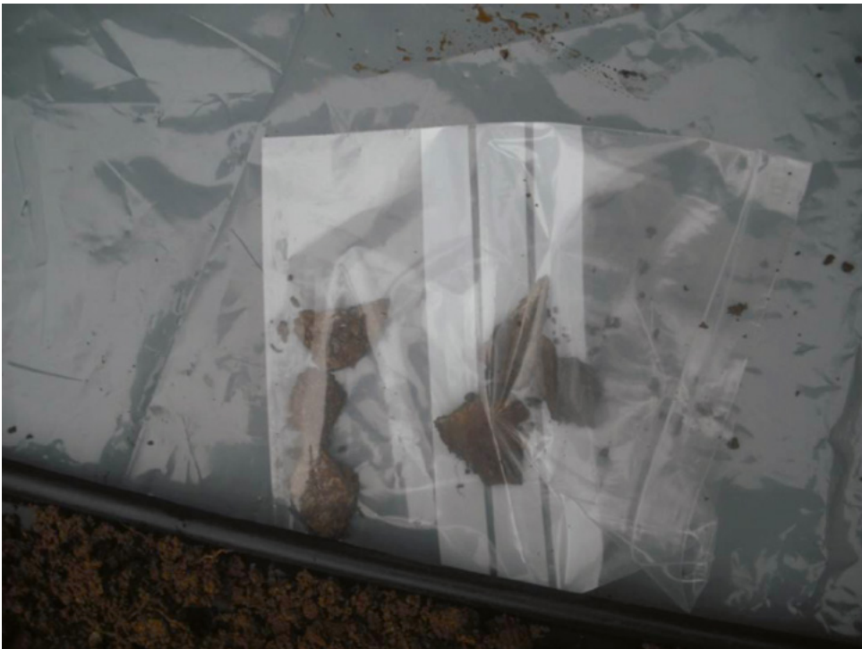
Figure A7.6 Examples of similar suspect ACM fragments picked out for cleaning and stereo-microscope examination. The three pieces to the right were confirmed as AC
