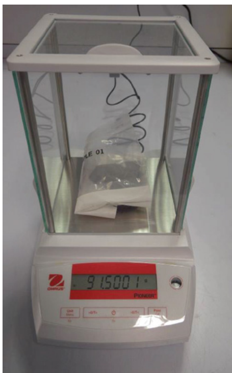
Figure A3.1 Water absorption sample being weighed
