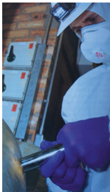
Figure 4.5 Analyst taking a core sample
