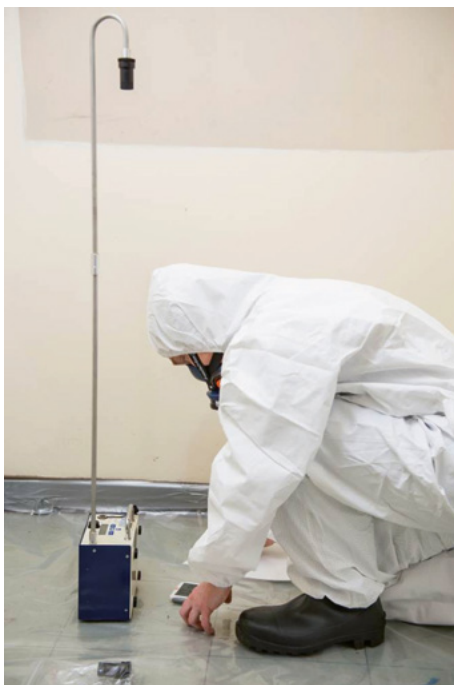
Figure 5.5 Analyst setting up a clearance test
