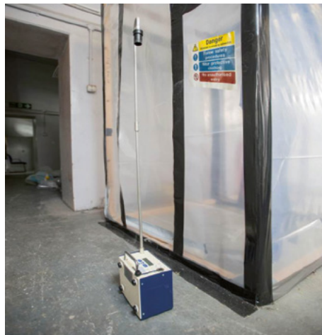
Figure 5.6 Leak test outside an airlock
