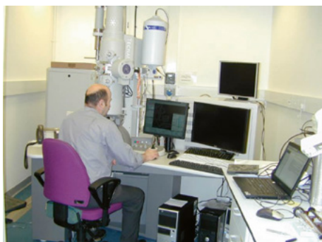
Figure A4.2 Transmission electron microscope in use
