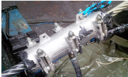
Figure 7: Typical Arrangement of Proprietary Pressurised Rope Lubrication Device
