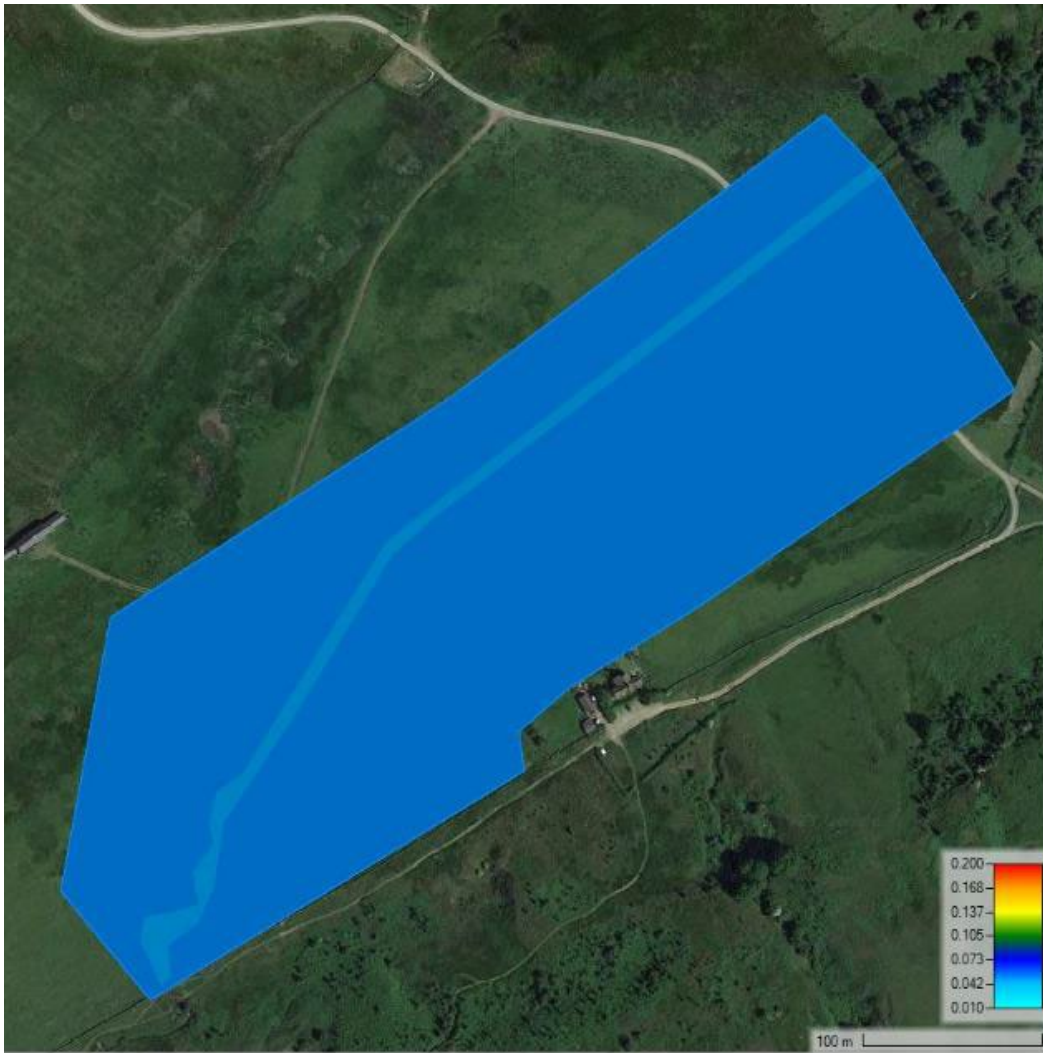
Figure 11.3 Baseline Manning's roughness grid.
