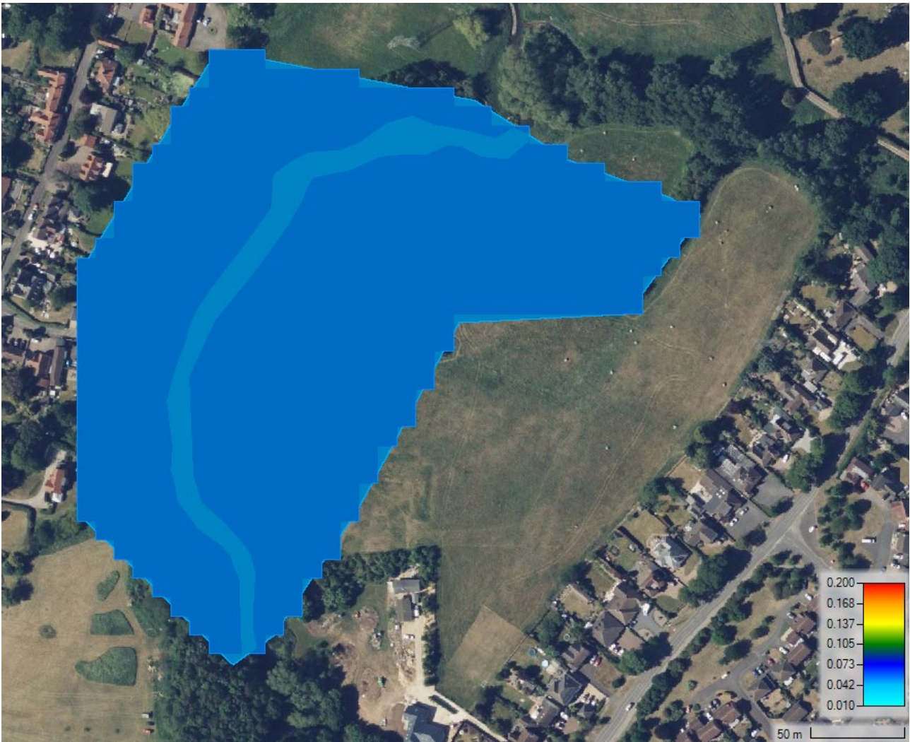
Figure 13.4 Baseline Manning's roughness grid.
