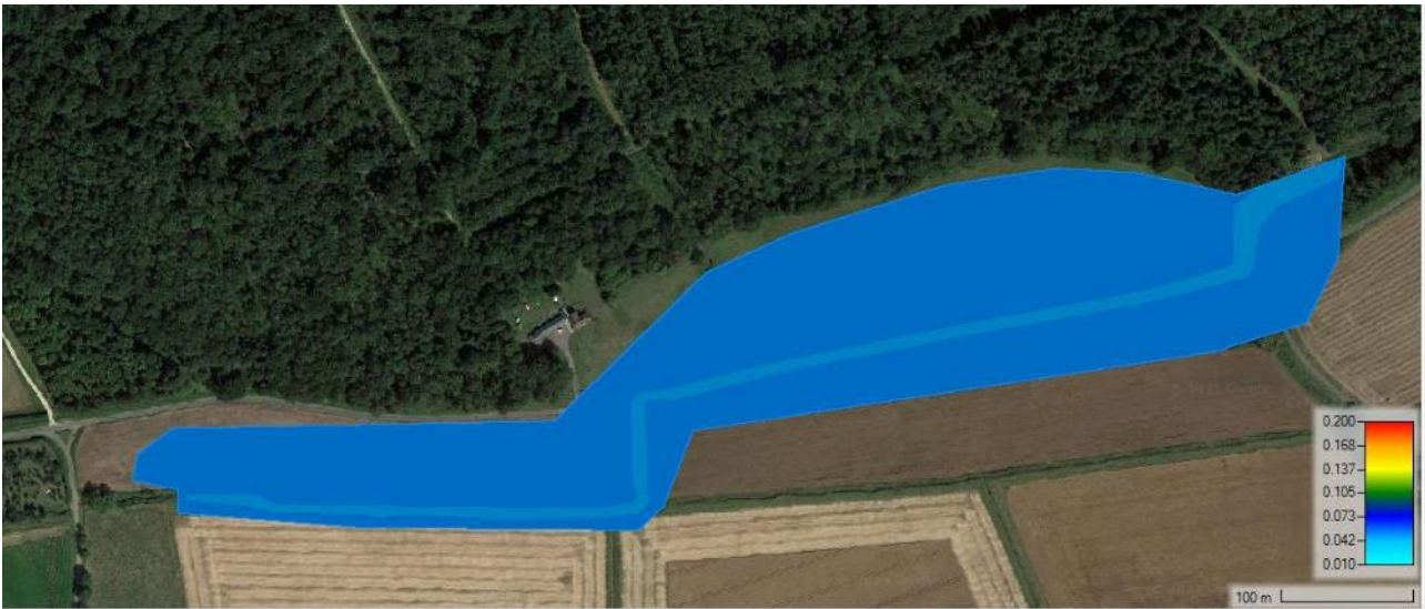
Figure 12.4 Baseline Manning’s roughness grid.
