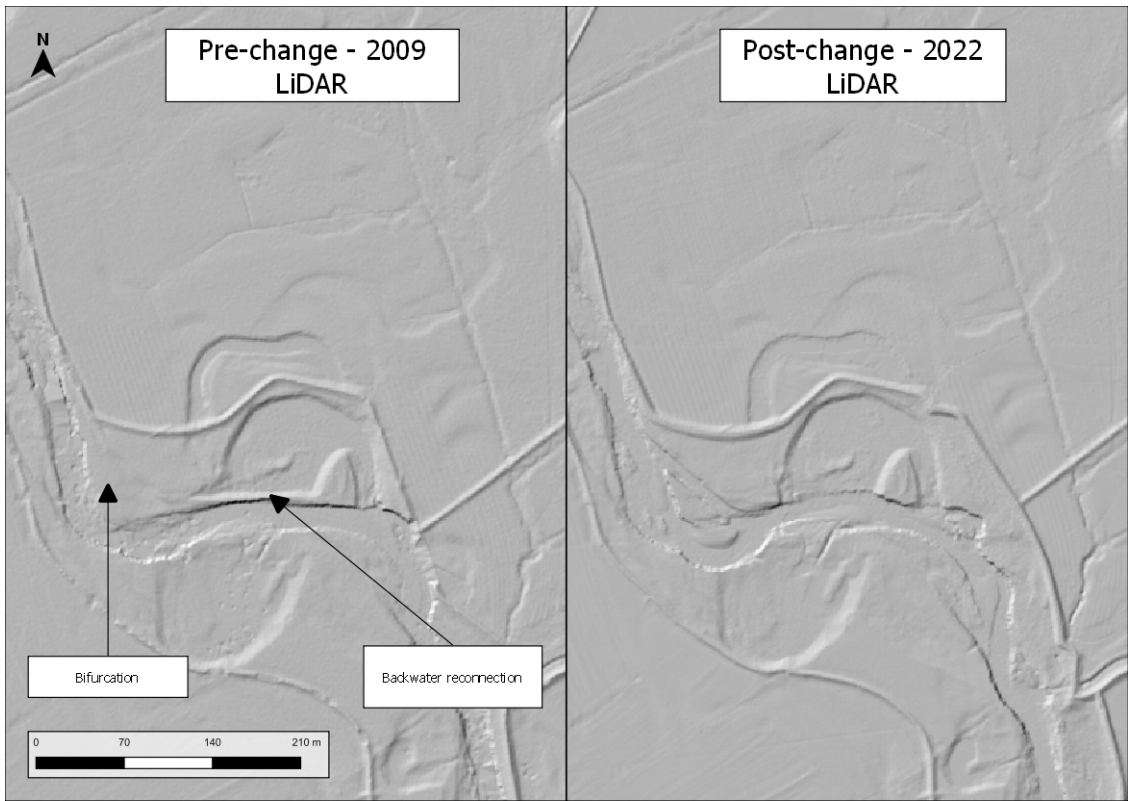
Figure 6.16 River channel pre (left) and post (right) bifurcation and backwater connection.
