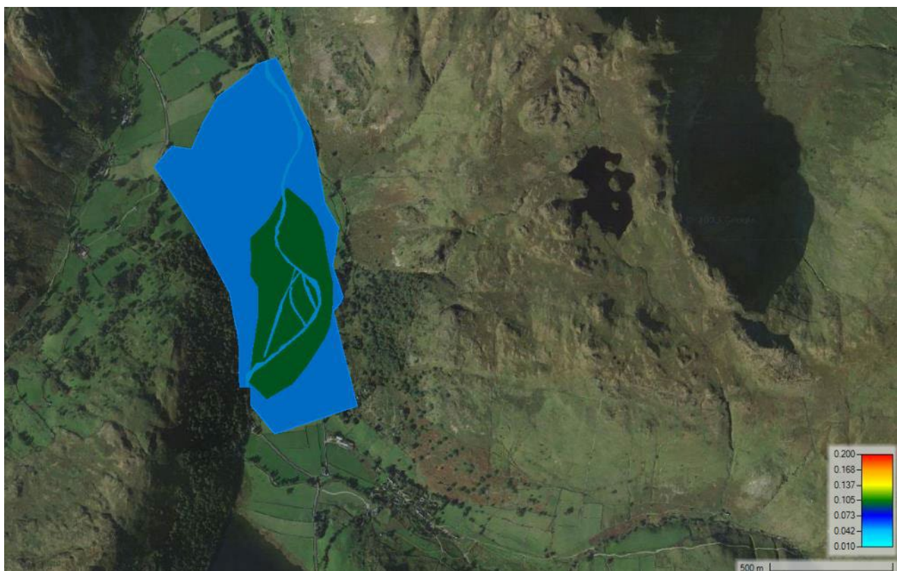
Figure 9.5 Post-change Manning's roughness grid
