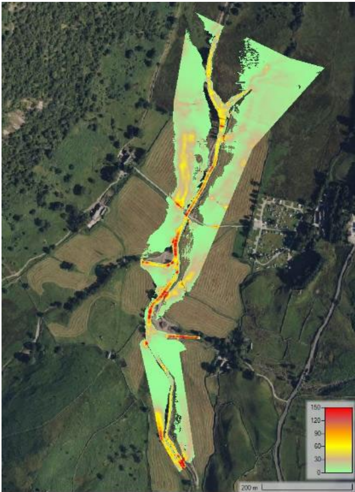
Figure 10.12 1 in 2yr bed shear stress pre-restoration.
