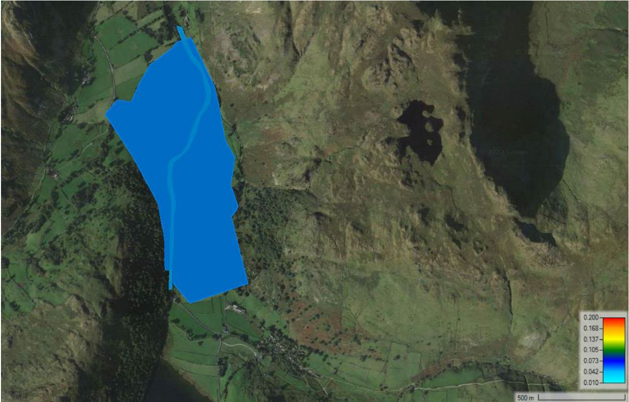
Figure 9.4 Baseline Manning's roughness Grid.
