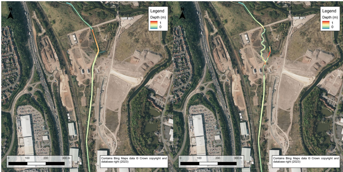
Figure 8.5 Pre (left) and post (right) change depths during Q10 flows.
