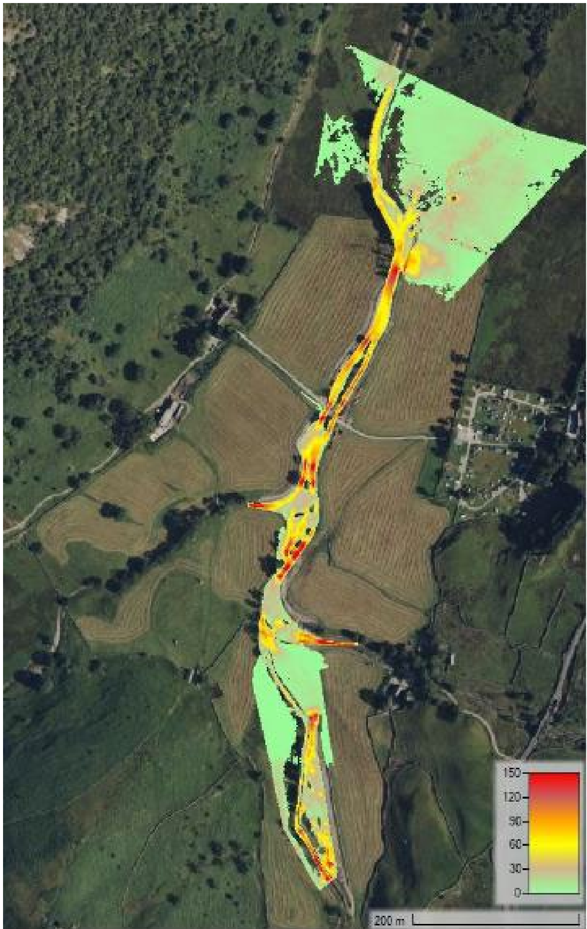
Figure 10.13 1 in 2yr bed shear stress post-restoration.
