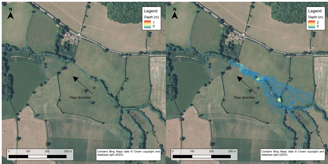
Figure 7.7 Depths for pre (left) and post (right) restoration scenarios during a Q95 flow.
