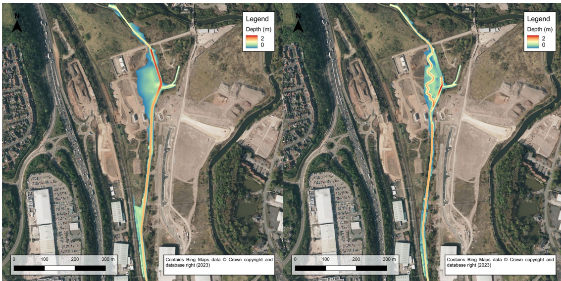
Figure 8.6 Pre (left) and post (right) change depths during a 2-year flood flow.
