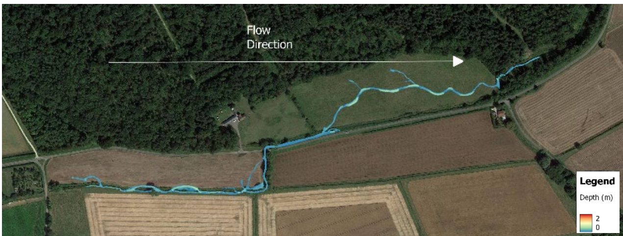
Figure 12.6 Water depth pre (top) and post (bottom) restoration scenarios for the Q95 flow.
