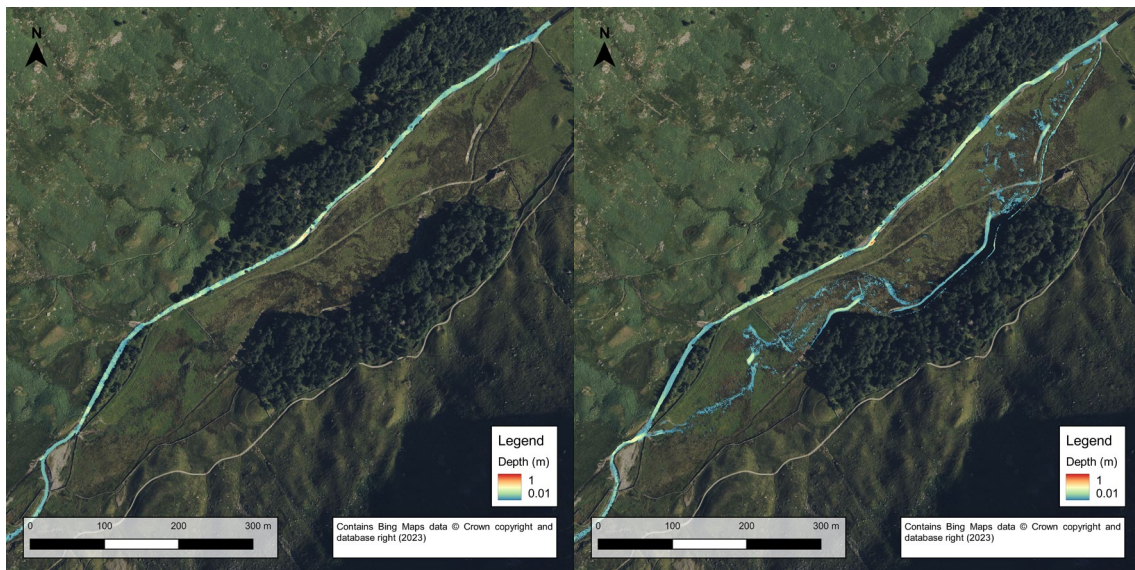
Figure 4.6. Post (left) and post (right) change depths during Q10 flow.
