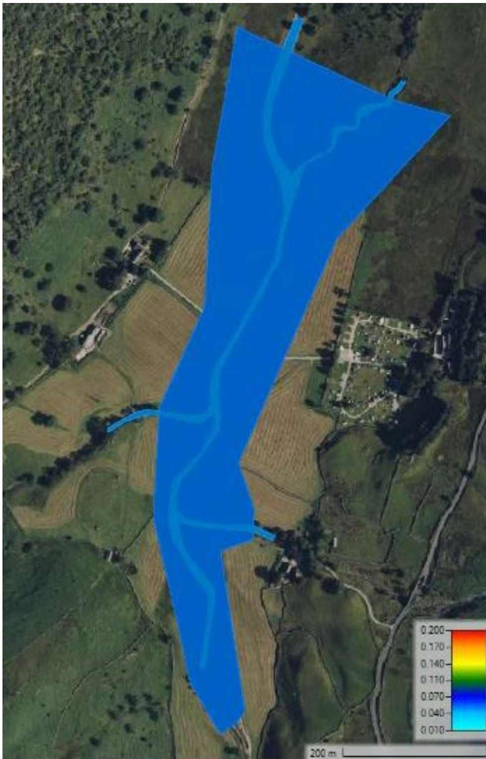
Figure 10.4 Baseline Manning's roughness Grid.
