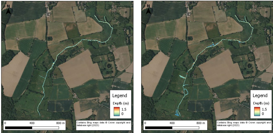
Figure 5.2 Depth pre and post restoration scenarios during Q95 flow.
