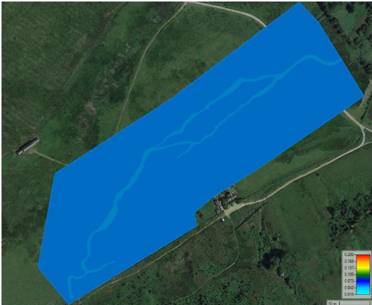
Figure 11.4 Post-change Manning's roughness grid.
