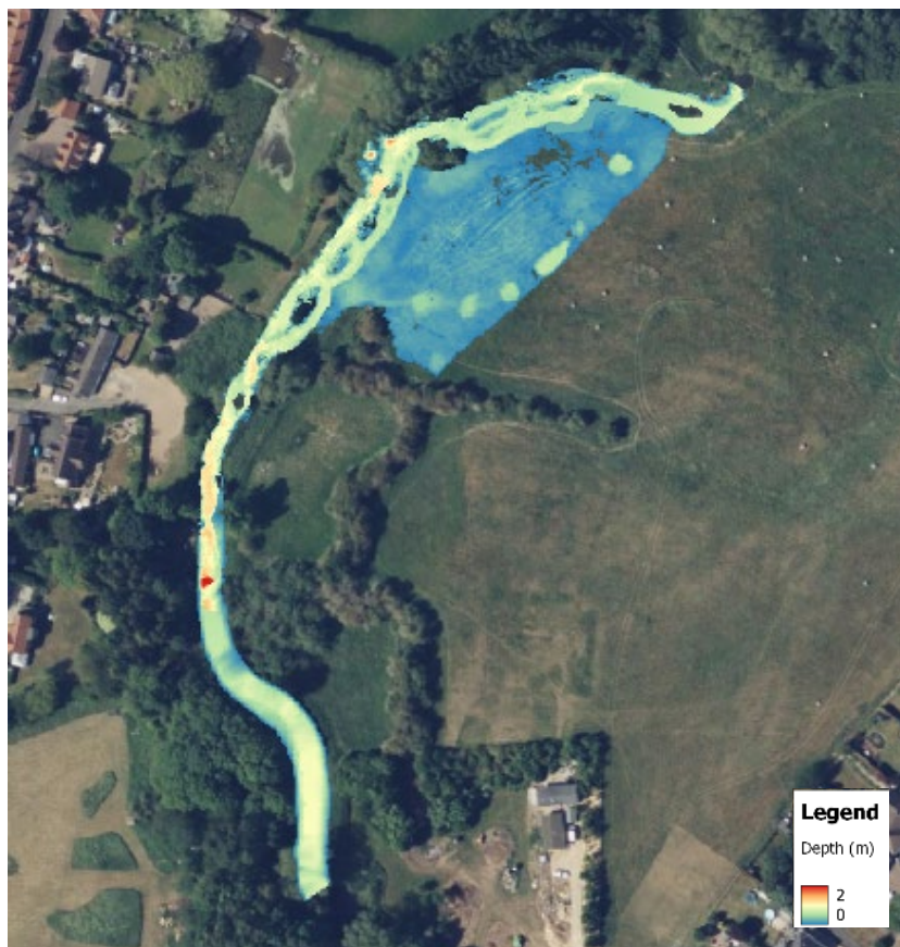
Figure 13.8 Water depth pre (top) and post (bottom) restoration scenarios for the 2-year flow.
