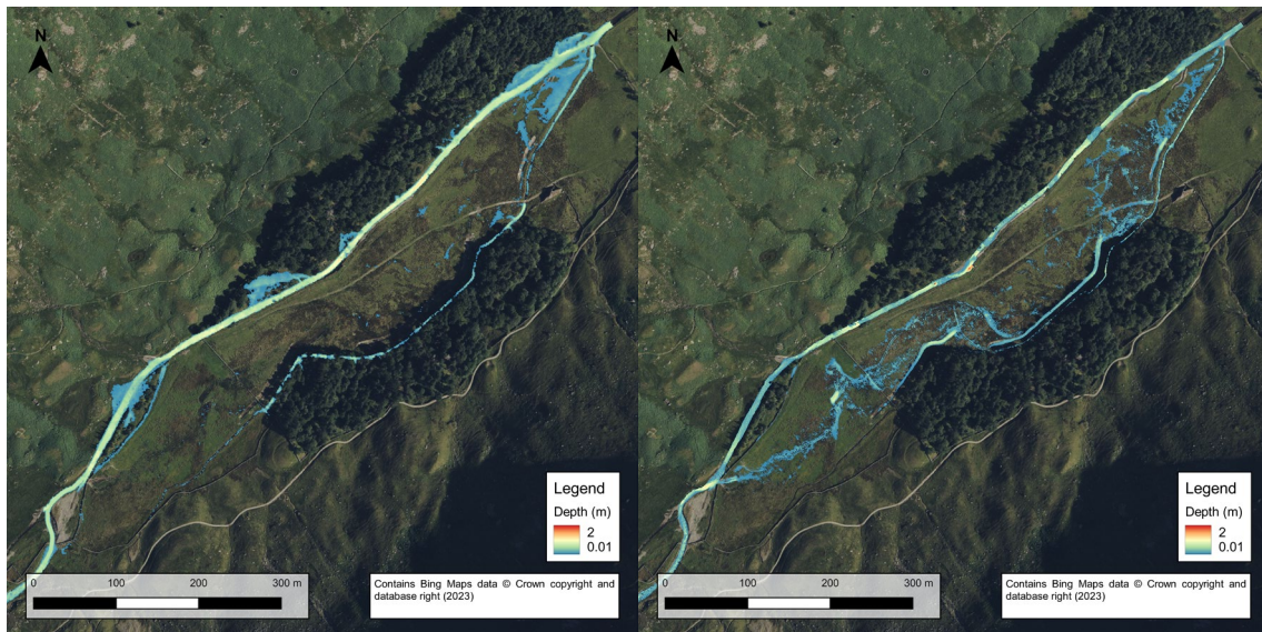
Figure 4.7. Post (left) and post (right) change depths during Q10 flow.
