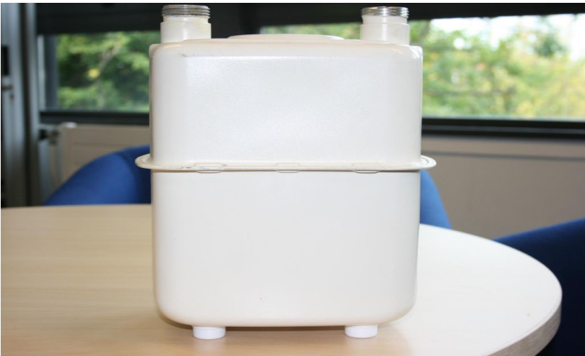
Gas meter – No rust over meter band
