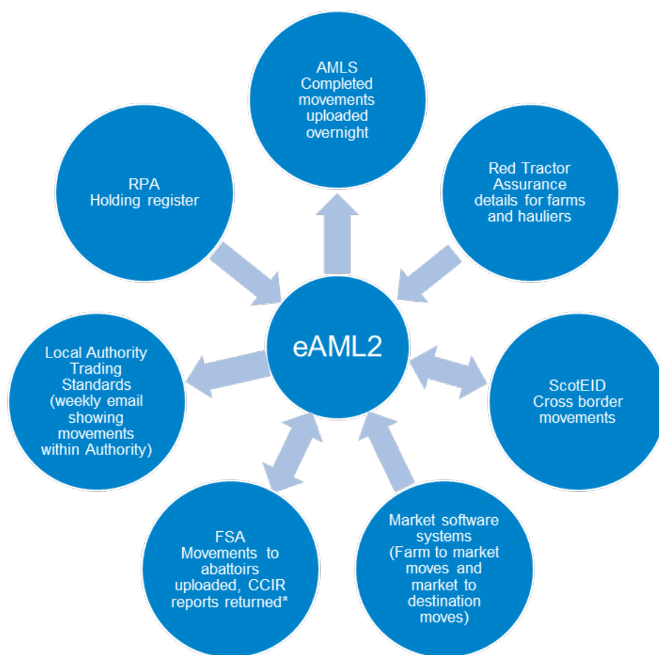
Figure 7: Demonstrating the external interfaces between eAML2 and other databases
