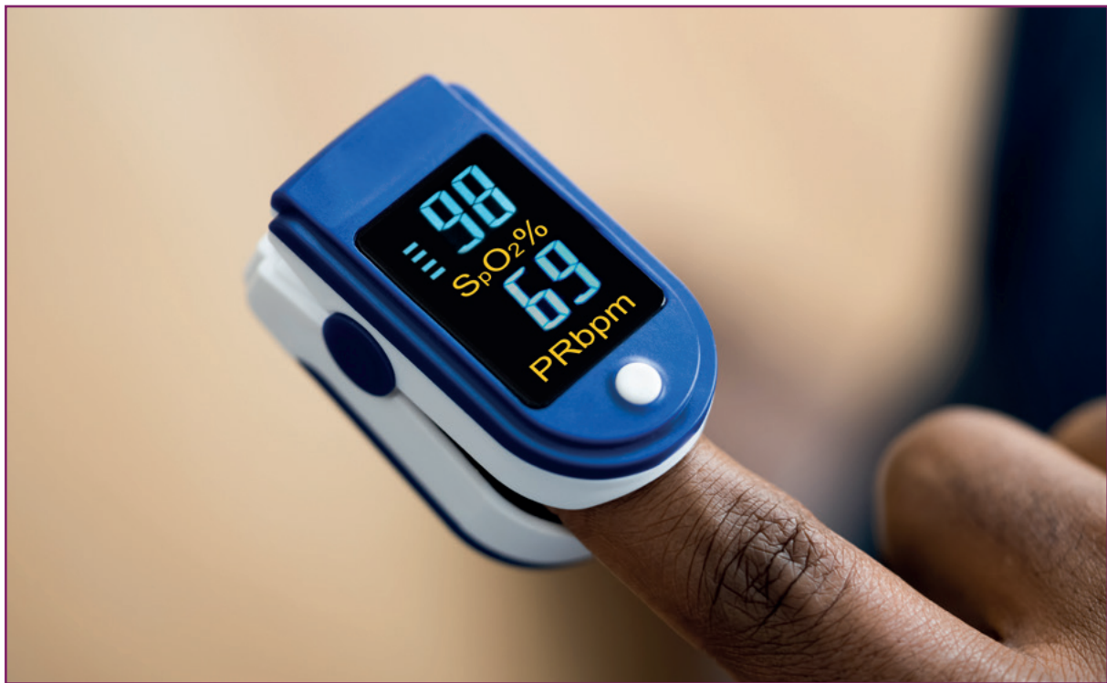
Figure 4: A battery-operated fingertip pulse oximeter
