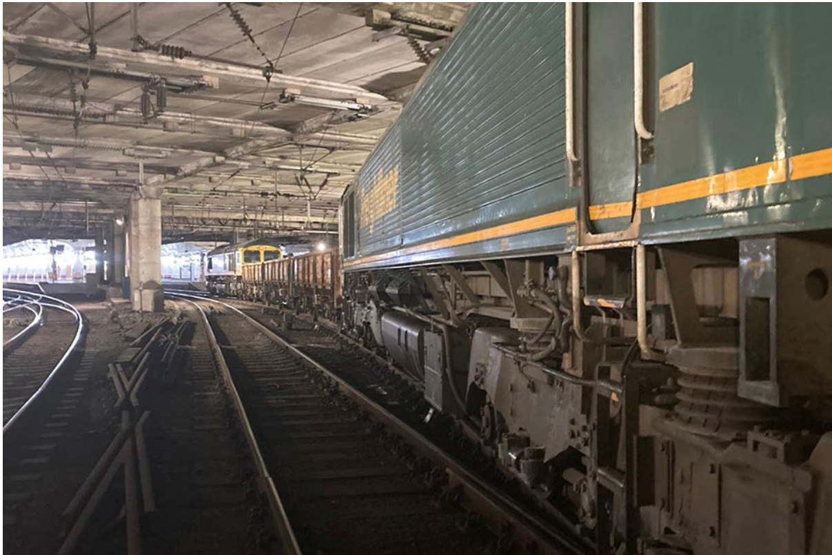
The position of the train on the set of trailing points as found afterwards (image looking back towards the station platform courtesy of Network Rail).
