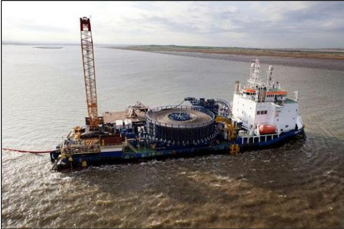
Figure 3.14: Example Of A Typical Cable Installation Vessel Showing The Cable Carousel On The Deck
